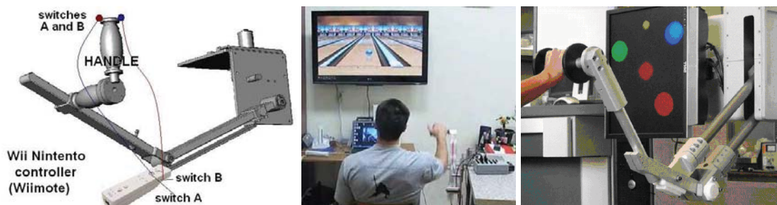
Figure 1: 2D pantograph with adaptable lengths of arms, remotely positioned switches A and B, and the Wiimote fixed to one arm of the pantograph (left panel), the pantograph in use for bowling game (middle panel), and Brachio di Ferro robot that is envisioned to be connected with the pantograph (e.g., the same handle) and used as the robot trainer (right panel).
