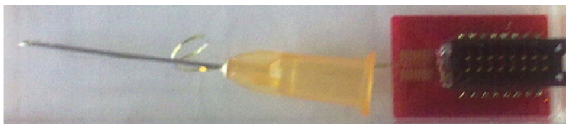
Figure 1: Thin-film electrode system with needle for insertion into the muscle and connector.
