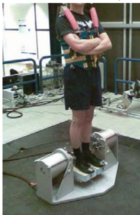
Figure 1: Left: a subject on the Bipedal Ankle Perturbator (BAP). The BAP consists of two support surfaces which can independently rotate in dorsi-/plantarflexion direction. The axes of rotation of BAP are aligned with the axes of rotation of the ankles. Right: typical response of a subject; the subject was instructed to lean forward. Solid lines show a condition in which the calf muscles are stretched (dorsi flexion); dashed: plantar flexion rotations ('unloading' the calf muscles).
